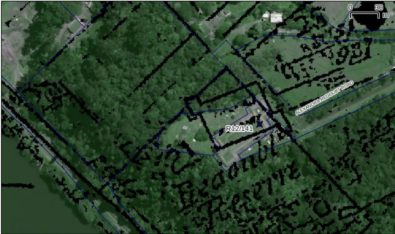
Figure 62 Detail from SO 413 of 1866, overlaid on 2012 aerial imagery, with the modern cadastral dataset as blue lines.
