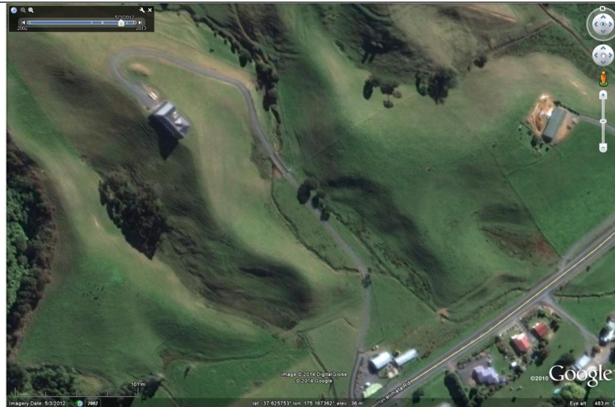
3. By May 2012 a house was relocated to the ridge. The image indicates that the driveway did not interfere with the toe of the slope, which subsequently failed in July 2012. The image also indicates that no earthworks were undertaken on the slope.
