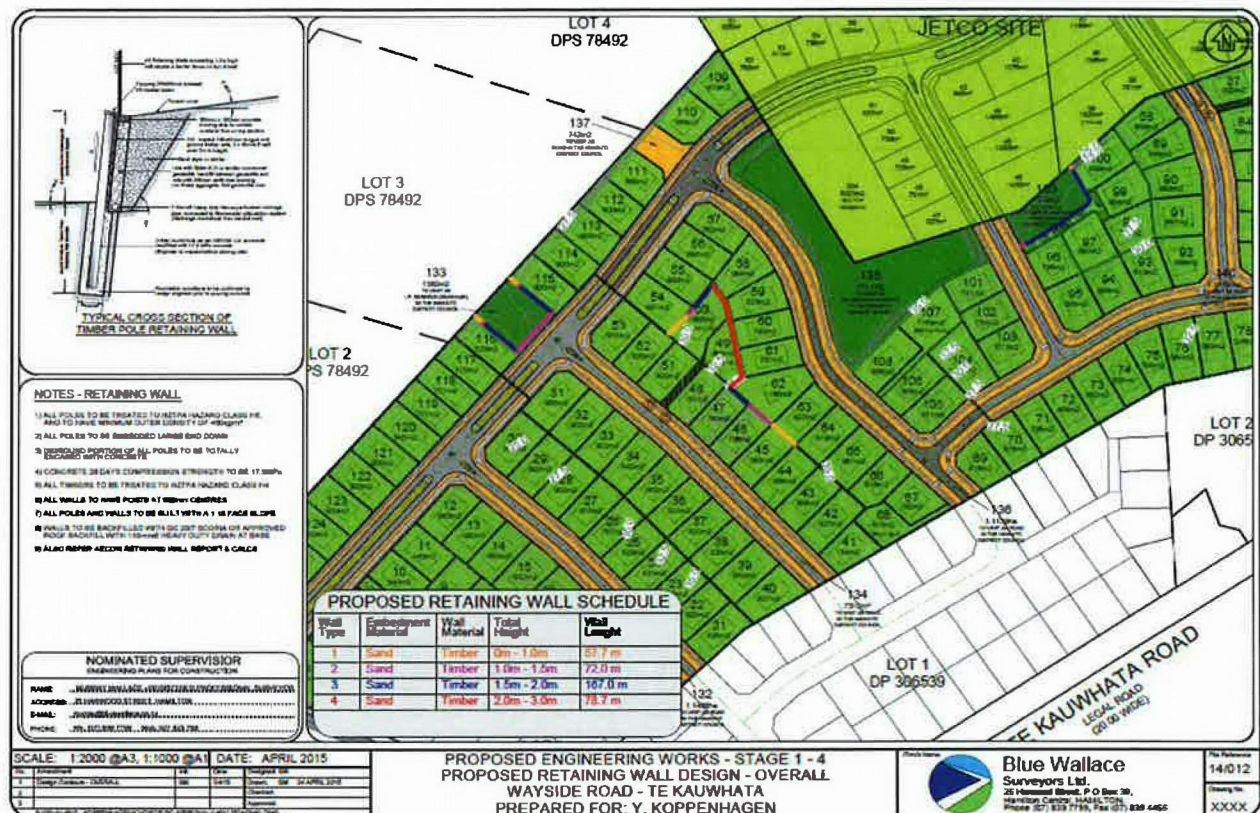
Image 3 – Retaining Wall Plan
