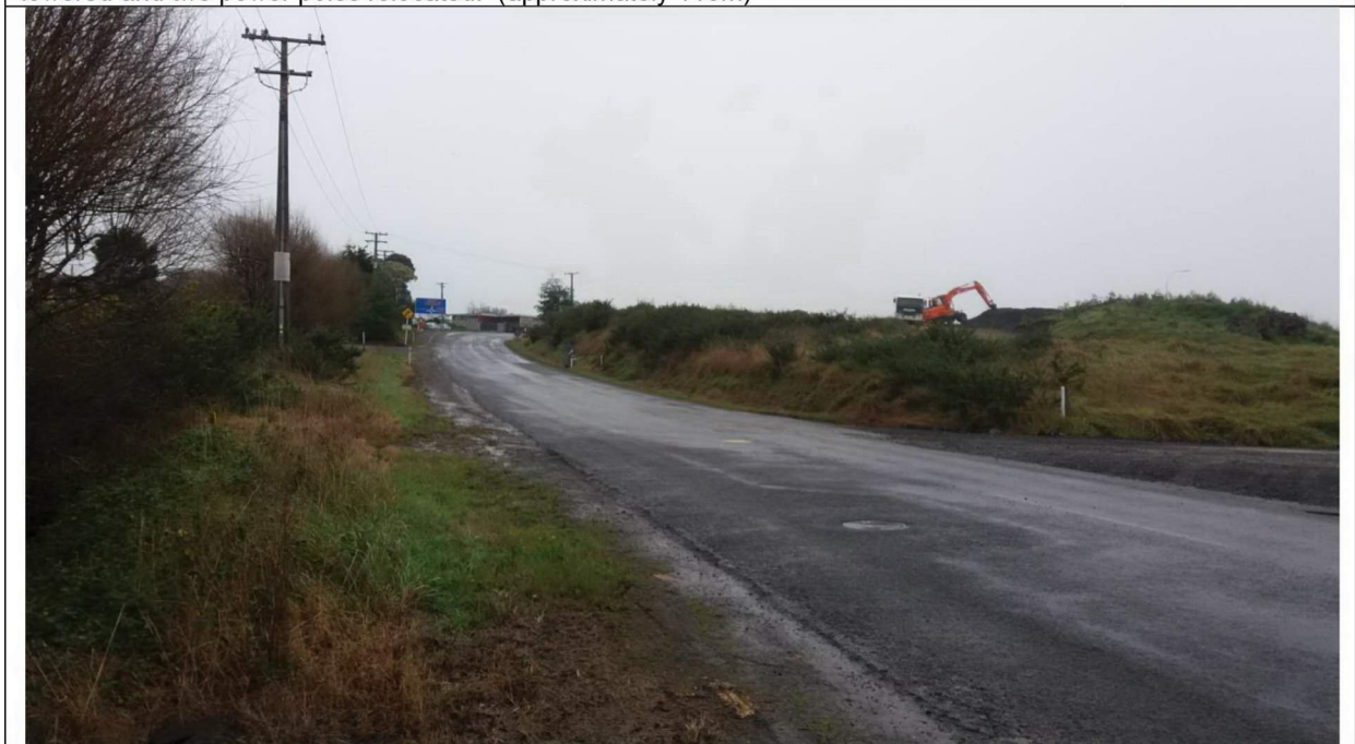
Photograph 4: Existing visibility to the south from the proposed intersection is approximately 210m. Note that the long section by Blue Wallace shows this as 195m.
