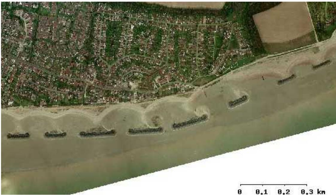
Figure 24: Breakwater Example at Elmer, UK (courtesy of Wikipedia)
