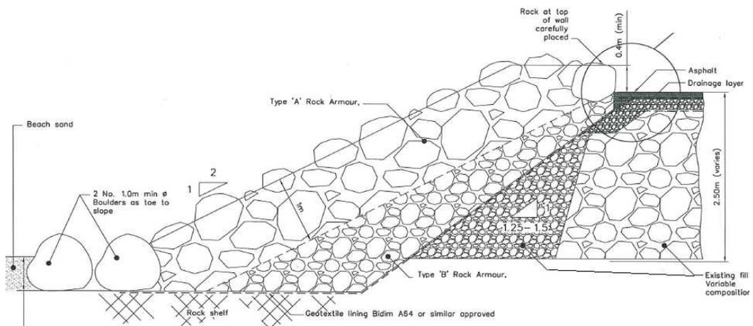
Figure 13: Profile of rock wall design (Source: Previous project by GHD)
