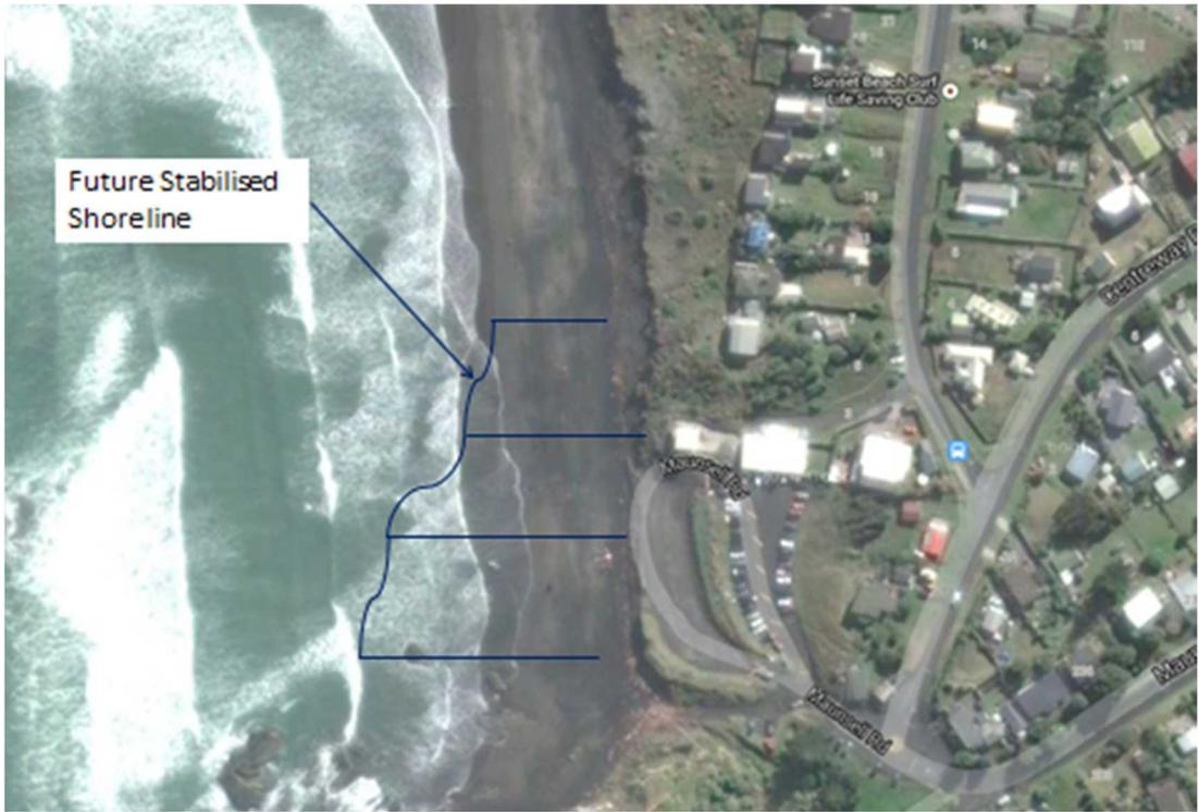
Figure 25 : Diagram of Potential Groins at Port Waikato
