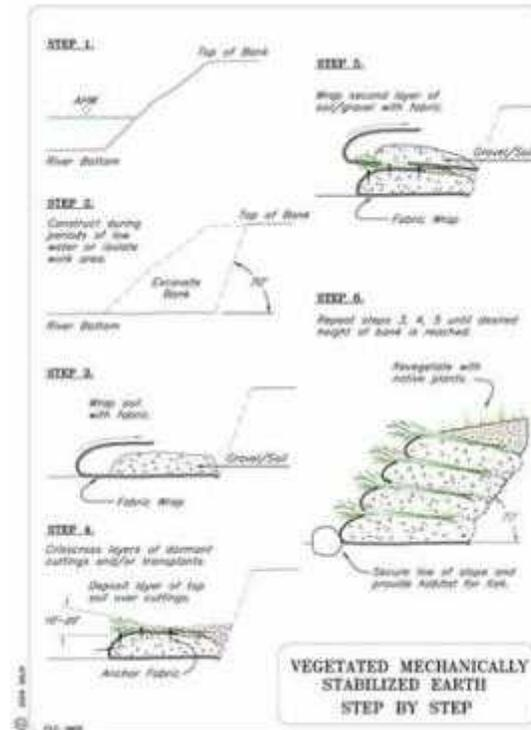
Figure 15: Wall design using geo fabric (Source: RST Solutions 2014)
