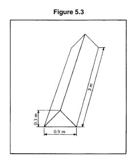
Moulded plastic markers filled with water - https://flightgse.com/product-lines/airfield-markers/
